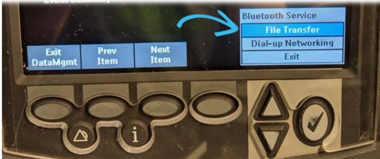
16. Once completed, a success message appears. Press the check mark button to acknowledge this message and then exit the *Bluetooth Device List* menu.
